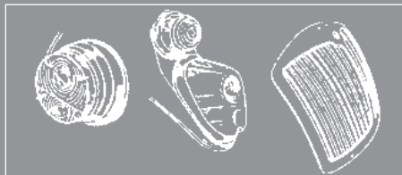
Front parking lamp lenses became 'flat' and a separate indicator lamp was added. The front grille on 1600cc models is identical to the 1500cc grille.
